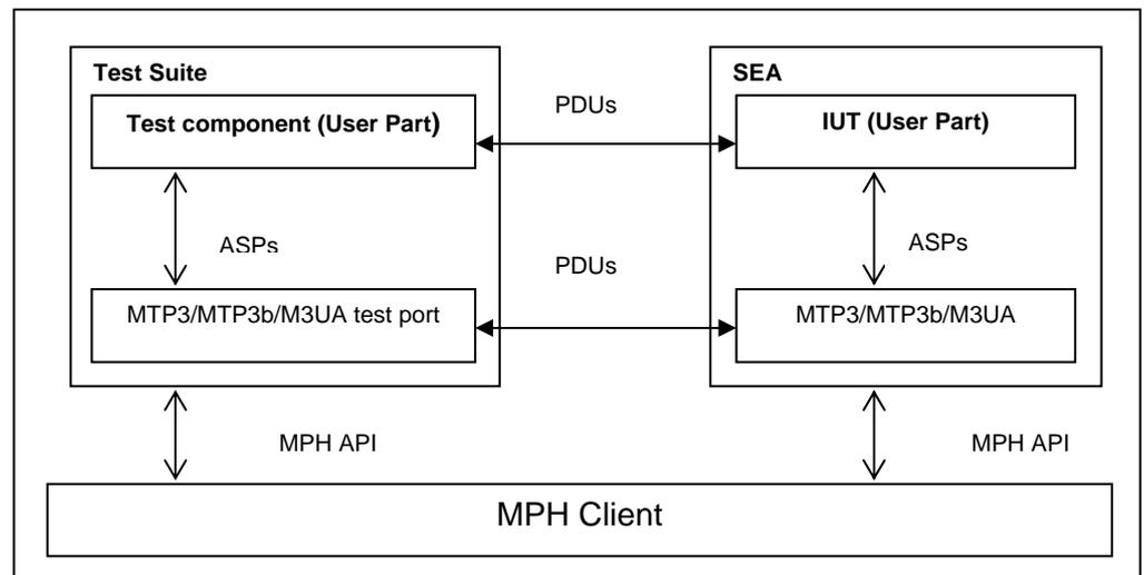
Figure 1 The overview of the test system using MTP3/MTP3b/M3UA test port
