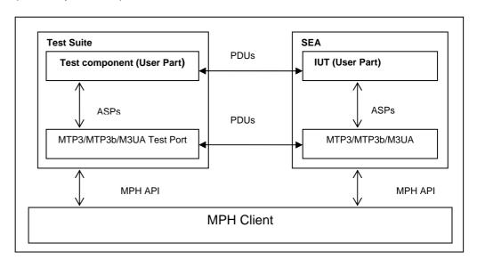
Table 1 The overview of the test system using MTP3/M3UA Test Port
